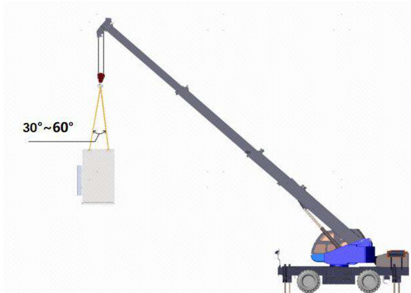
Figure 6-10: Crane lifting(for reference only)
